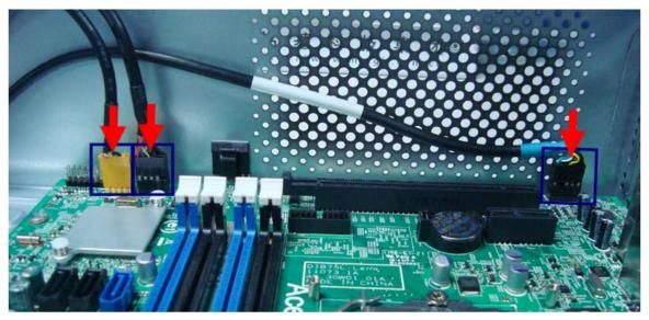
4. Install the retention clip to chassis, then install the front audio cable into the plastic clip.
